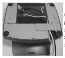
Place all the cables required for connections to the TP6000 series except those for special application purposes into the cable passage. Inset one end of the cable passage cover under the battery cover and screw on the two screws. Be sure not to damage any of the cables during this operation.
